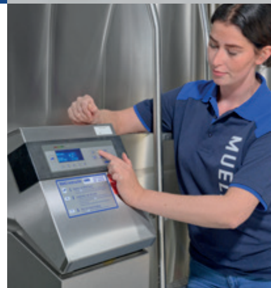
MIII Control Unit Large display showing milk temperature, date, time and system information in several languages
